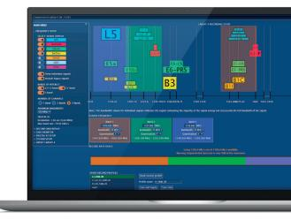
The interface's customisation extends to each RF channel, both in the pre-record phase and during replay, providing users the ability to adjust critical settings such as quantization, centre frequency, bandwidth, and sampling rate.
